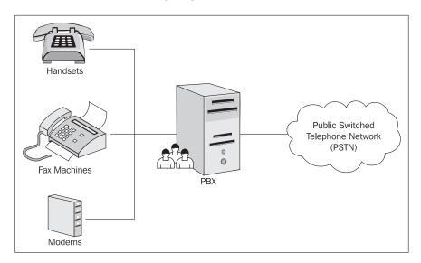
In this diagram, each extension (meaning everything to the left of the PBX) can connect to any other extension by dialing it directly. This means that if a modem were to send a fax to a local fax machine, it would be done by creating a direct connection between the devices through the PBX.
